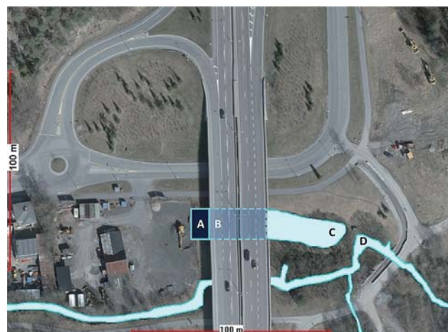
Fig. 1 Overview of the Skullerud sedimentation pond including parts of the catchment area and the recipient River Ljanselva: A = closed pre-sedimentation basin, B = pond inlet (PI), C = pond outlet (PO) and D = stream water (SW) upstream the pond outlet.
