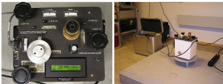
Figure A.2: LaCoste & Romberg relative spring gravimeter of the G-type with the ALIOD100 upgrade. (Photo: Kristian Breili)
