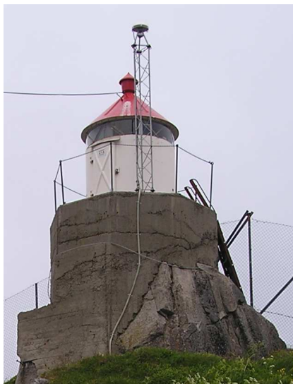
Figure 4.6: The GPS antenna at Honningsvåg is placed close to the lighthouse with its characteristic sloping roof covered by plates of metal. Multipath signals from this roof are likely to be the origin of the strong signal with a period of 11.97 h found in the GPS height series.
