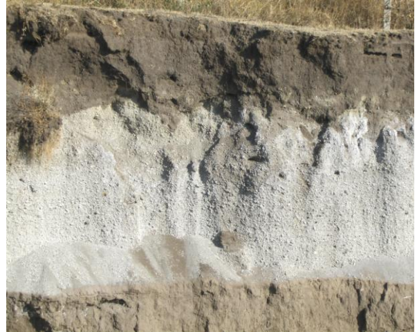
Plate VI: Volcanic ash (pumice soil) along the sides of Awassa Shashemene highway, Southern Ethiopia
