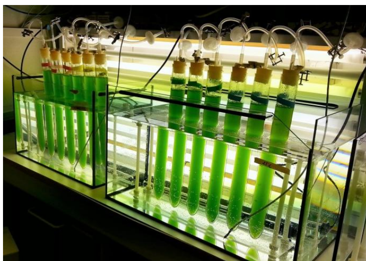
Figure 18. Photobioreactors used for batch cultures of C. reinhardtii . Photo: Marit E. Evjen.
