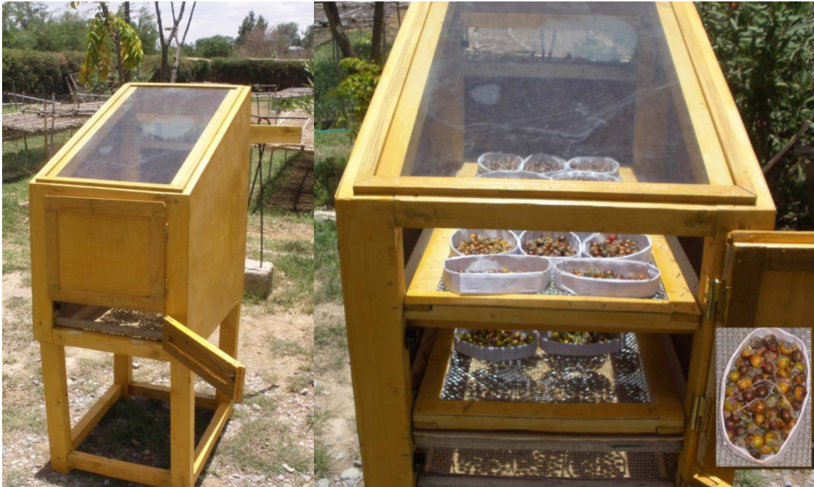
Figure 8. Box or cabinet direct solar drier and singular different coloured thread marked fruits in the drying process.
