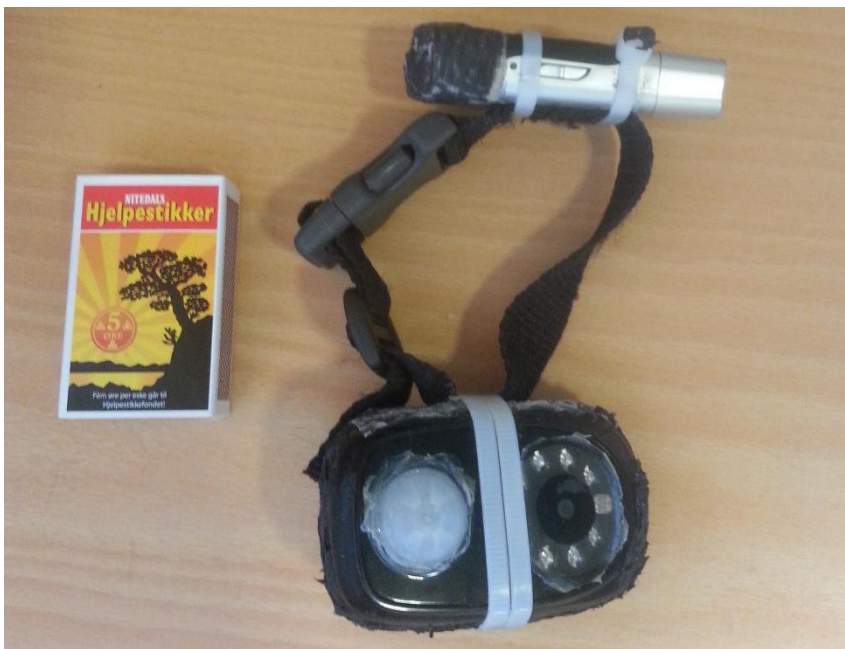
Figure 2. The collar used in the study. The GPS device mounted above the neck, and the camera below. The matchbox is included in the image to give a size reference (L x W x D = 80 mm x 40 mm x 25 mm).
