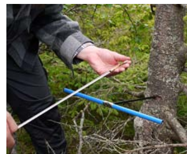
Figure 3 – Sample being taken with increment borer.
