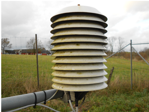
(a) The Vaisala HMP35D in a radiation shield Vaisala DTR13
