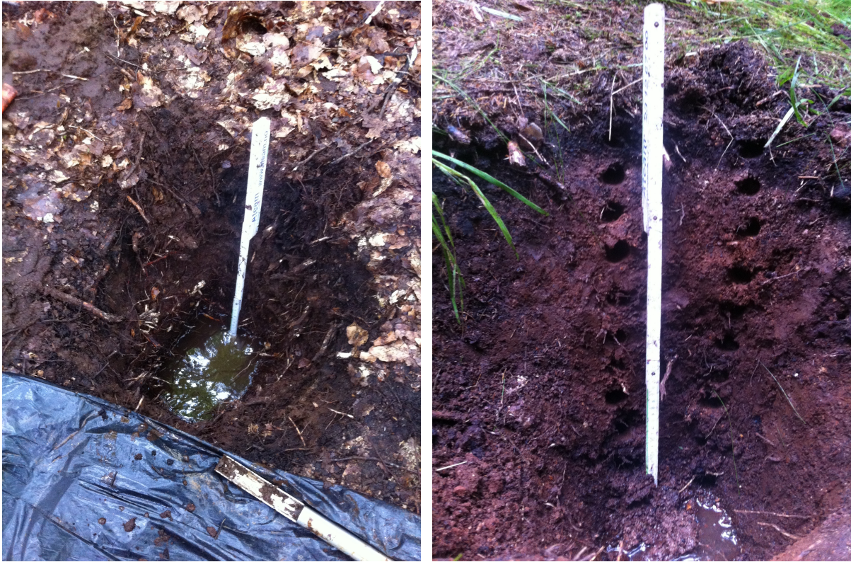
Figure 4: Illustration photo from two of the sampling plots, one of the beech forest (A3) (left) and the other of the first-generation spruce forest (B3) (right). In the foreground of the photo on the left, from the beech forest, lays the steel cylinder used to collect soil samples.
