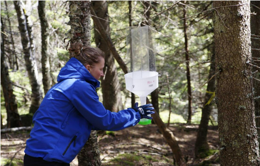
Figure 2.3: Window traps. Four window traps were used in each site. The traps were hung between two tree trunks, with a distance of 0.5 m to each tree and 1.5 m to the ground. The traps consisted of two crosswise acrylic panes (40 x 22 cm) leading down to a funnel with a 0.5 litre bottle attached to it. The bottle was filled with 2 dl of propyleneglycol with water and a dash of dishwasher soap.
