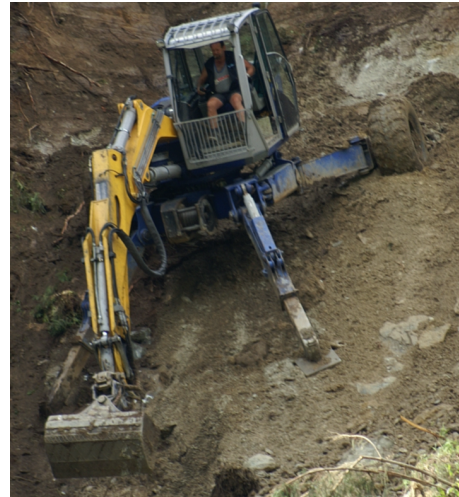
Figure 3.6: All terrain excavator. Photo by Böhlinger Friedrich, via Wikimedia Commons
