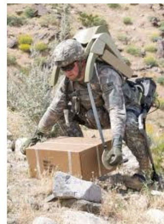
Figure 2.16: Lockheed Martins HULC exoskeleton with Lift Assist Device. Photo by permission from Lockheed Martin.
