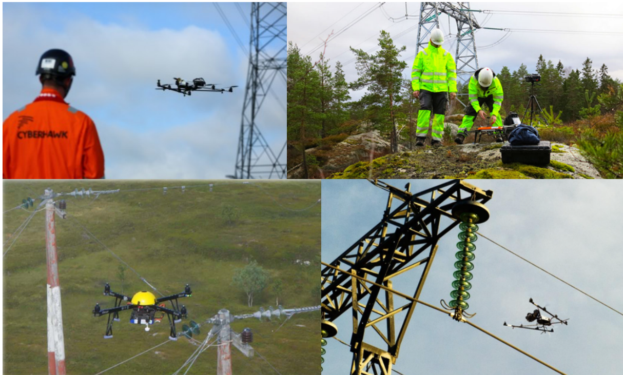
Figure 2.7: Up left: Cyberhawk performing aerial inspection of a transmission tower using an UAV. Photo by permission of Cyberhawk.
