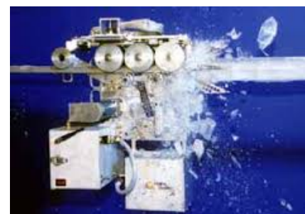
Figure 2.4: LineROVer by Hydro-Québec de-icing a ground wire. Photo by permission from Hydro-Québec.
