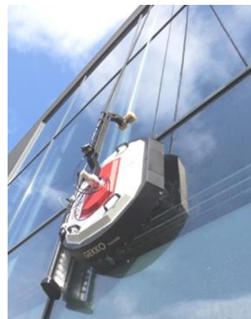
Figure 2.15: GEKKO Facade performing window cleaning. The robot is fastened with a rope from the top of the building. Photo by permission of SERBOT AG
