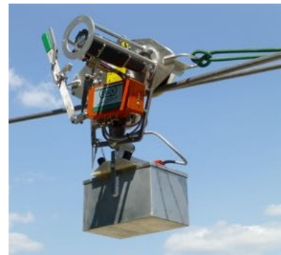
Figure 2.3: LKE 85 Pulling robot for replacement of ground wires. Photo by permission of Zeck.
