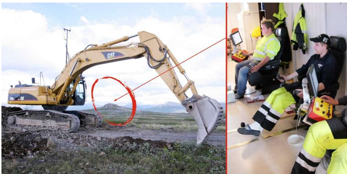
Figure 2.11: Operators from Gjermundshaug Anlegg AS remotely controlling construction machinery from the marked hilltop in the background. Photo: © Harald Grevskott, Vi Menn Magazine.
