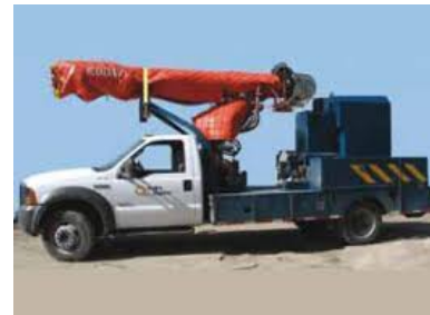
Figure 2.10: Remotely Operated De-icing All-weather Vehicle by Hydro-Québec. Photo by permission of Hydro-Québec.
