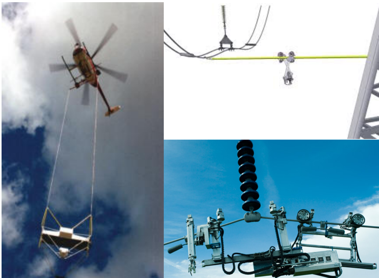
Figure 2.5: Left: Power Inspection Sweden's ROBHOT™ for measuring electrical resistance in phase conductor joints under live conditions. Photo by permission from Power Inspection Sweden AB Top right: Transmission Line Inspection Robot from Transpower New Zealand Ltd. Image by permission from Transpower. Down right: LineScout from Hydro-Québec crossing an insulator string. Photo by permission from Hydro-Québec.
