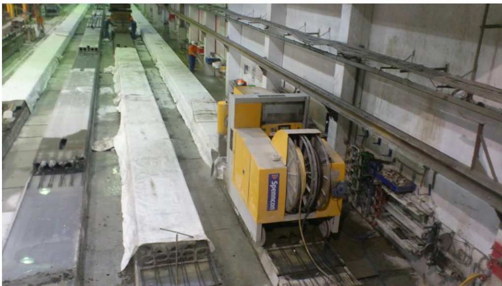
Figure 2-14: Machin that maces hollow core elements, picture from a tour at Spenncon in Hjoerungavaag
