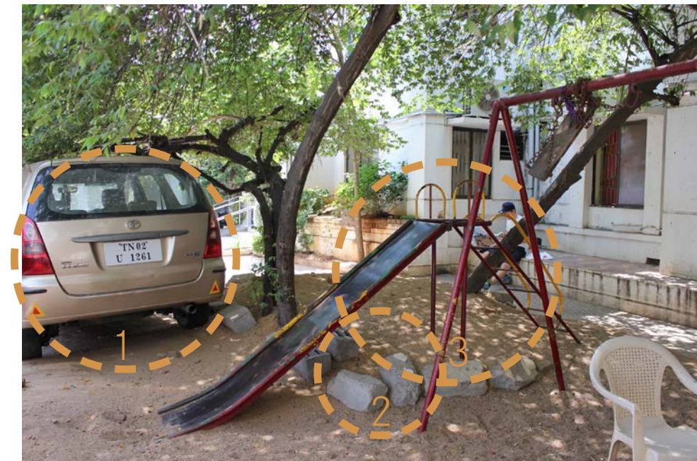
1. Cars are parked in the play area. 2. Rocks under the play equipment. 3. Safety zone overlap.
