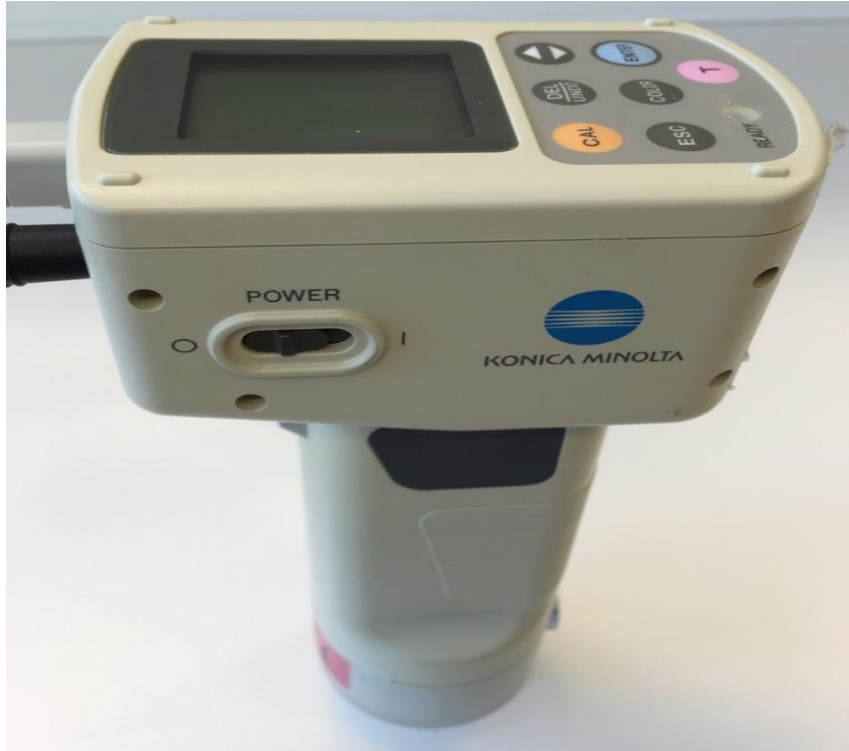
Figure 3.4: Konica Minolta CR400 Chroma Meter used for colorimetric analysis of dark spots on Day 0 and Day 7 post mortem.
