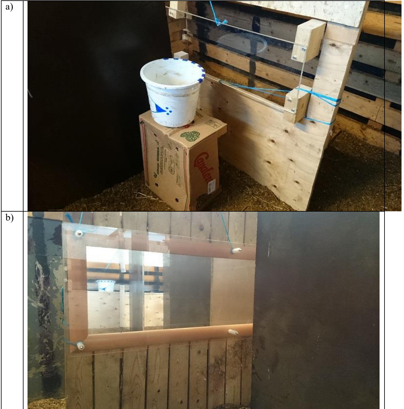
Fig.A.7. Example of (a) a glare in the window with a little bit of reflection from the bucket, (b) mirror-reflection of the window with the bucket behind.
