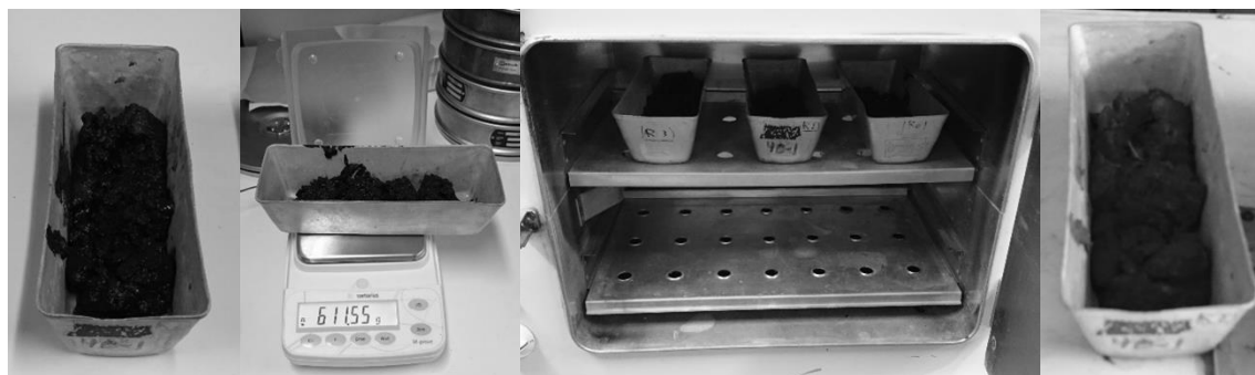
Figure 16. Weighing of samples before and after before and after drying
