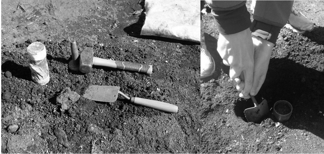
Figure 9. Collection equipment and techniques of soil sampling
