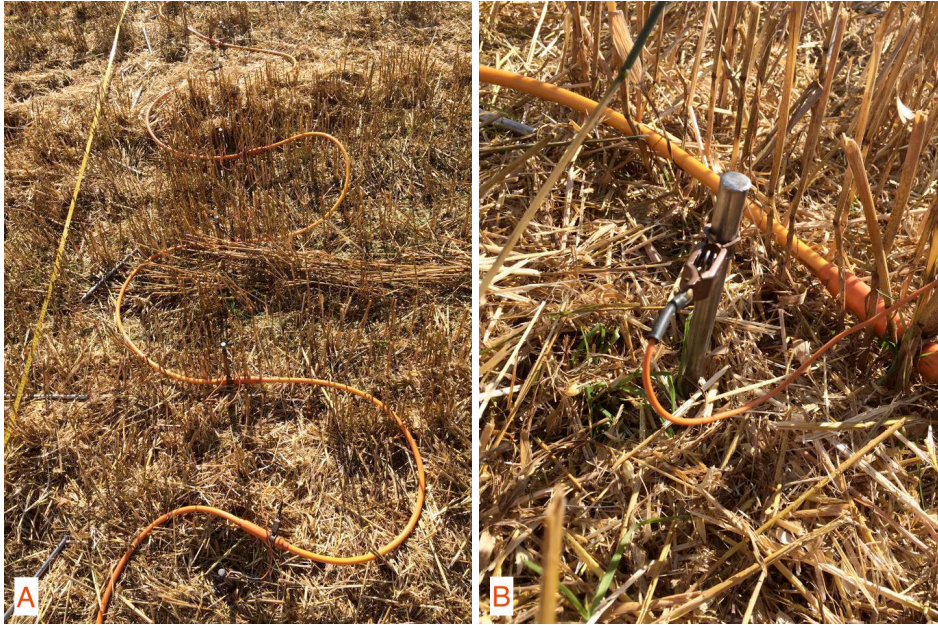
Figure 4-2: Image (A) shows how the ERT cable had to be laid out for the electrodes to have a spacing of 0.5 meters and (B) shows an electrode and how it is connected to the cable. Photo: Andrea Nymo Fikse.
