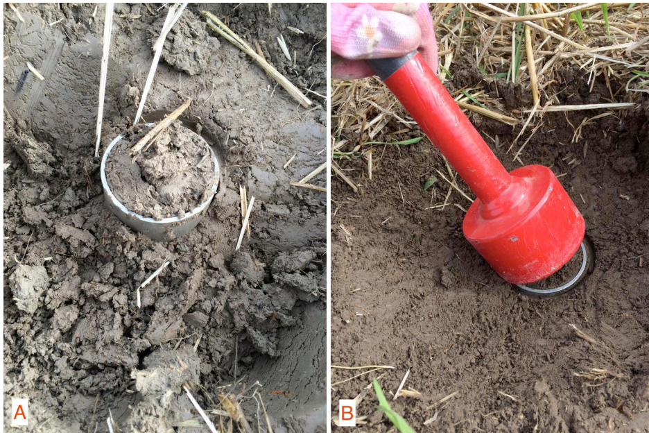
Figure 4-7: The steel cylinder had to be completely filled with soil, as shown in (A). To achieve this, a hammering head, as is shown in (B), was put on top of the ring before applying a hammer to beat the ring into the ground. Photo: Andrea Nymo Fikse
