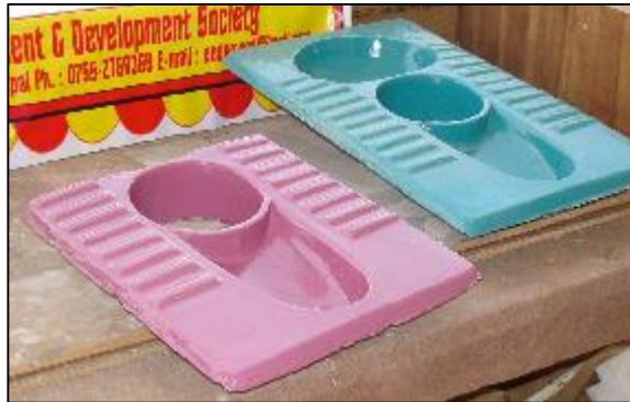
Figure 42 - Urine-diversion pans: the pink pan is for wet toilets and the blue pan is for dry toilets, with a separate hole for anal-cleansing water (Saxena 2009)
