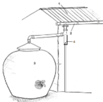
Figure 24 - Simple household rainwater system (Modified from Worm and Hattum 2006 to include first flush system)
