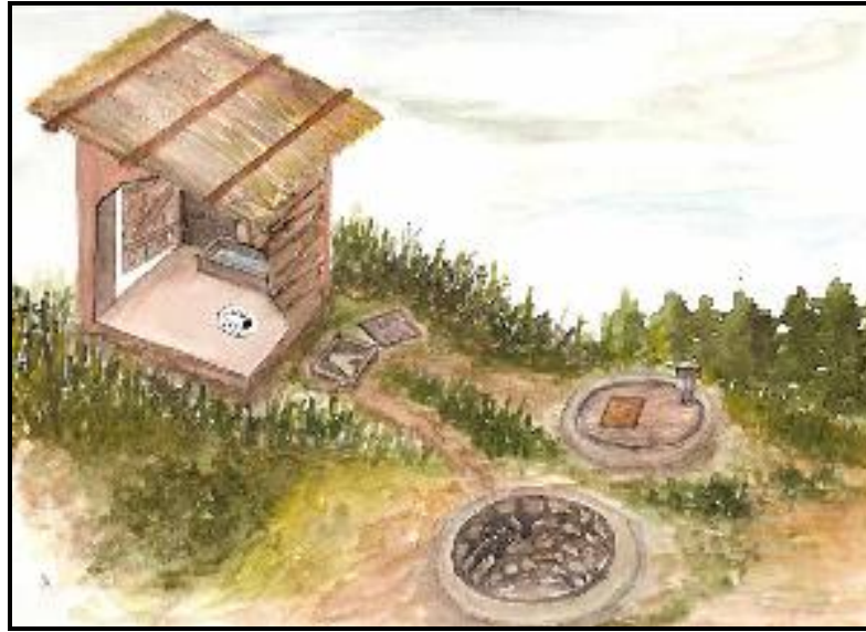
Figure 45 - Twin pit pour-flush latrine (Barun 2010)
