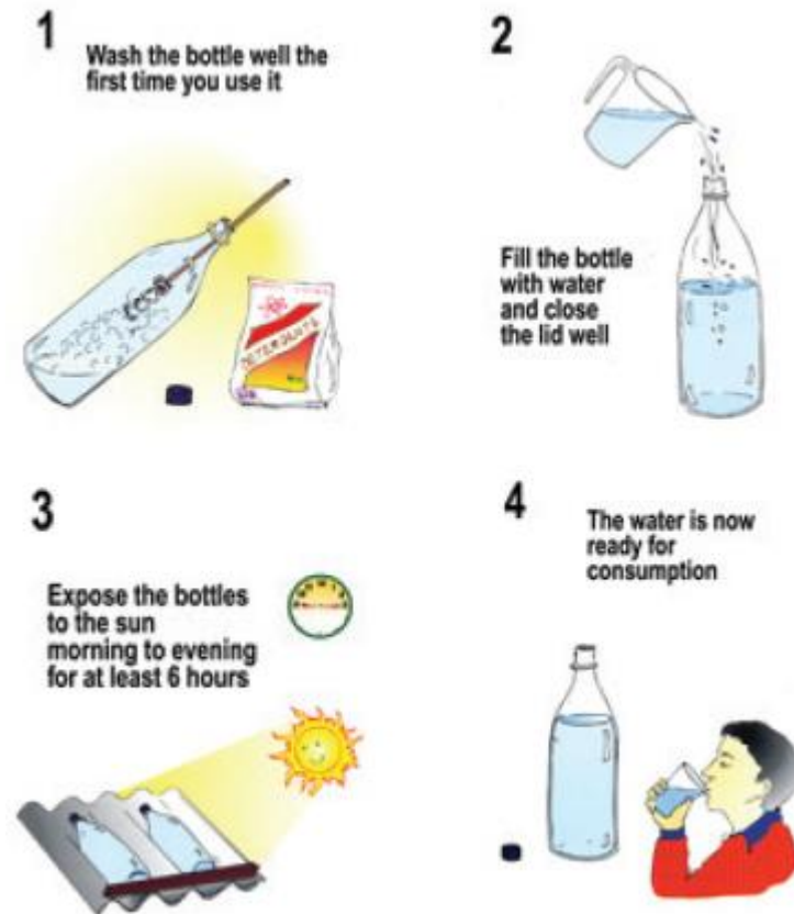
Figure 33 - Steps of the SODIS method (Luzi et al. 2016)
