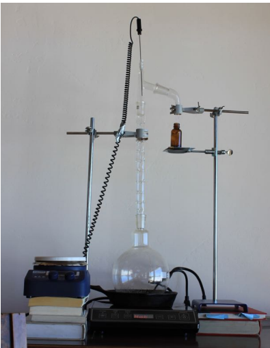
Figure 25 Fractional distillation apparatus (not set up for vacuum use)
