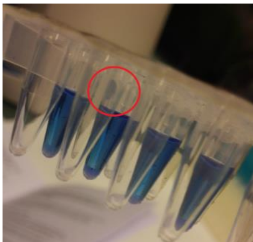
Figure 14 - Picture of the observed dry pellet along the wall of the sample well of RA5111B CD8. The red ring marks the dry pellet.
