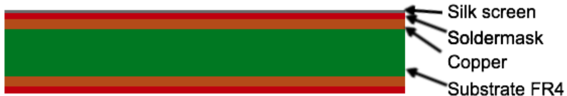
Figure 2-18: The layers of a PCB
