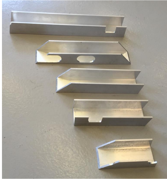
(b) All the U-beams
