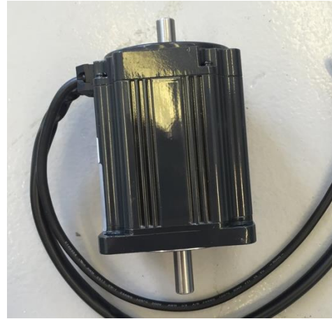
(b) Side-view to see the modified shaft
