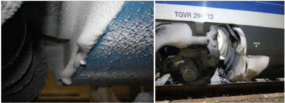
Fig. 24. Snow accumulation in the bogie cavity (wind tunnel model and real TGV train)
