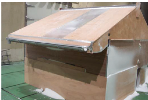
Fig. 10. Wind tunnel test of snow ingress through ventilated roof eaves
