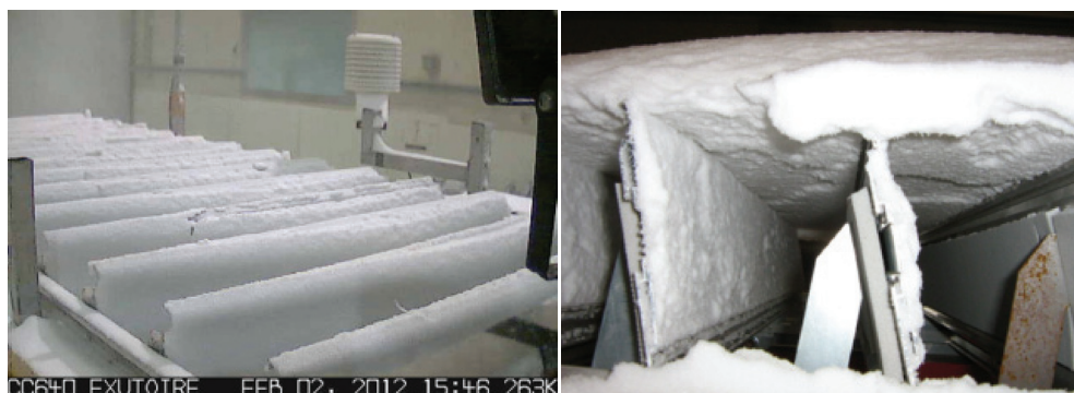
Fig. 16. Smoke vent opening test with snow loads
