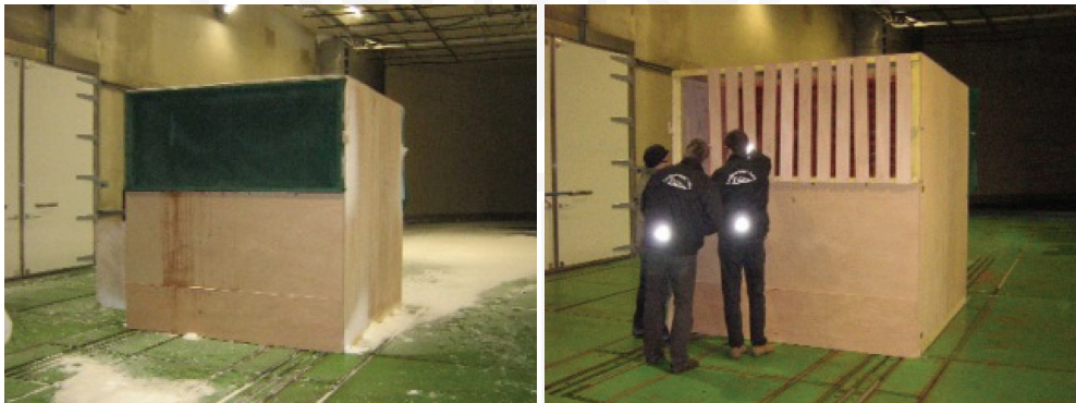
Fig. 3. Comparative testing of various air inlet snow traps in the wind tunnel
