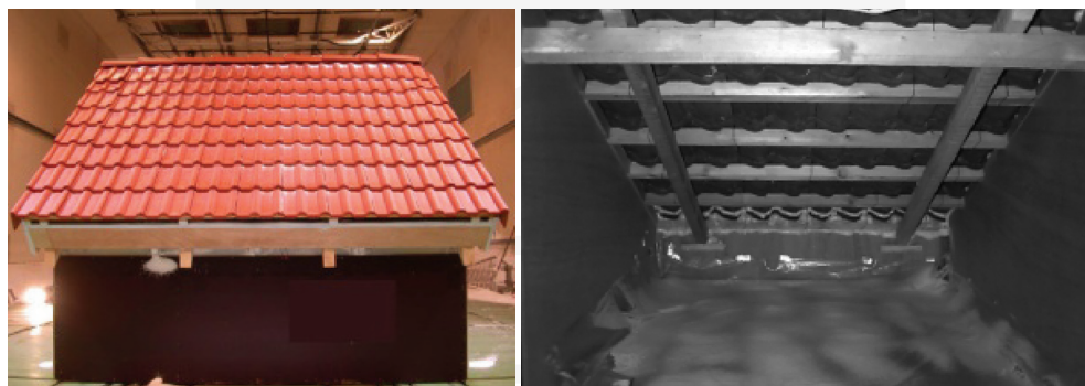
Fig. 8. Snow ingress between tiles in the model attic
