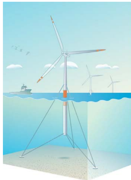
Figure 1. Artists impression of the TLB Baseline (B) conceptual design. The figure does not include the “crow-foot” deltas providing yaw stiffness
