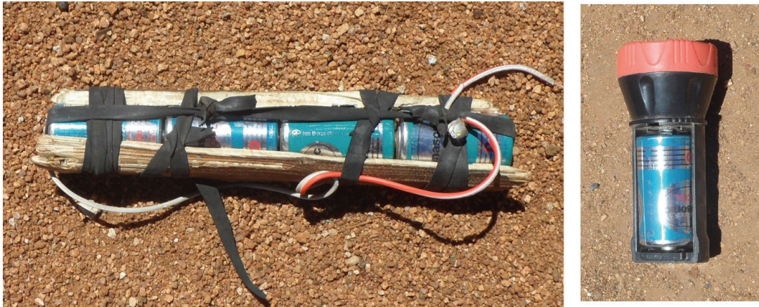
Plate 1 Dry cells in series used to make Richmond 2 left, and on the right, a common simple one-dry cell torch. Source: Author
