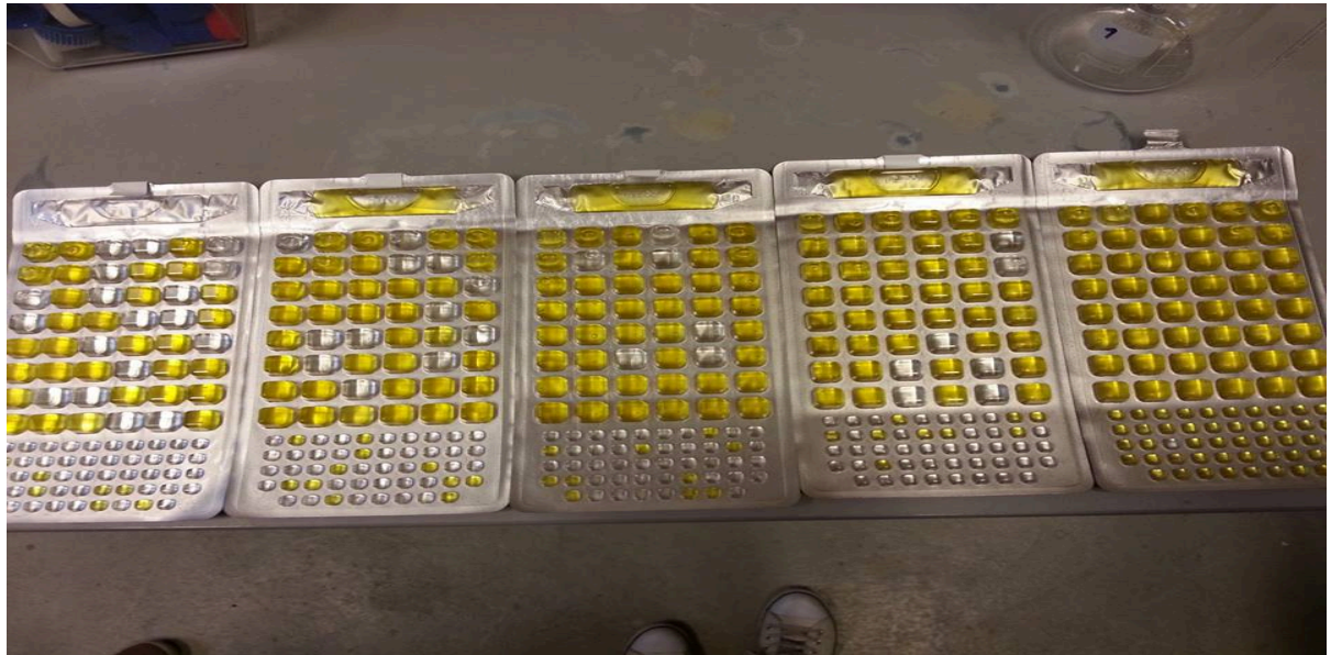
Figure 8.1 Quanti trays showing positive large and small well yellow pockets for coliform bacteria from day 0 laboratory experiments. (Silva 2015)
