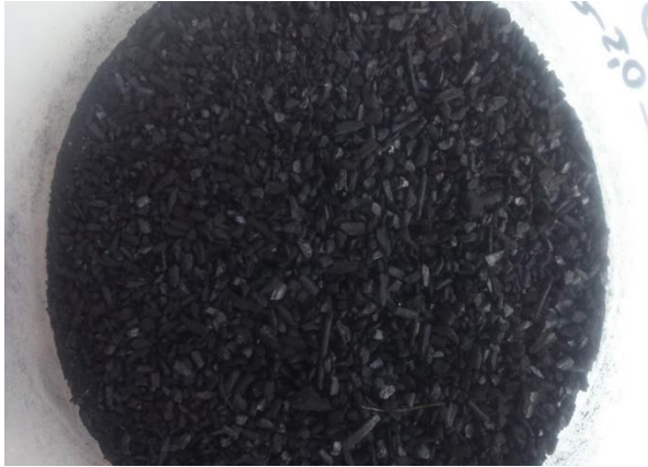
Figure 8 Woodchips biochar, pyrolysis at 480 °C.
