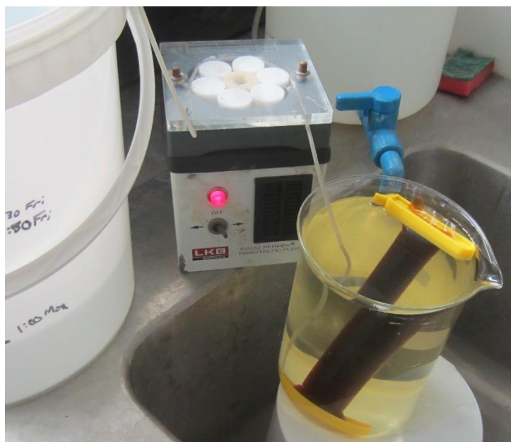
Figure 13 Dialysis phase of the DOC extraction process. A peristaltic pump provides a steady flow of fresh DW across a dialysis membrane used to filter forest litter extracts contained inside (dark liquid). Samples of the yellowish solution outside of the membrane were tested for electrical conductivity until stabilizing around 3 \mu\text{S cm}^{-1} .
