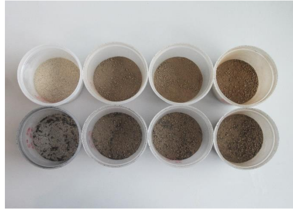
Figure 9 Vineyard soils used for experiments with 3% (w/w) biochar amended samples directly below (from left to right: Sand, Rossatz, Harm, and Stroh).
