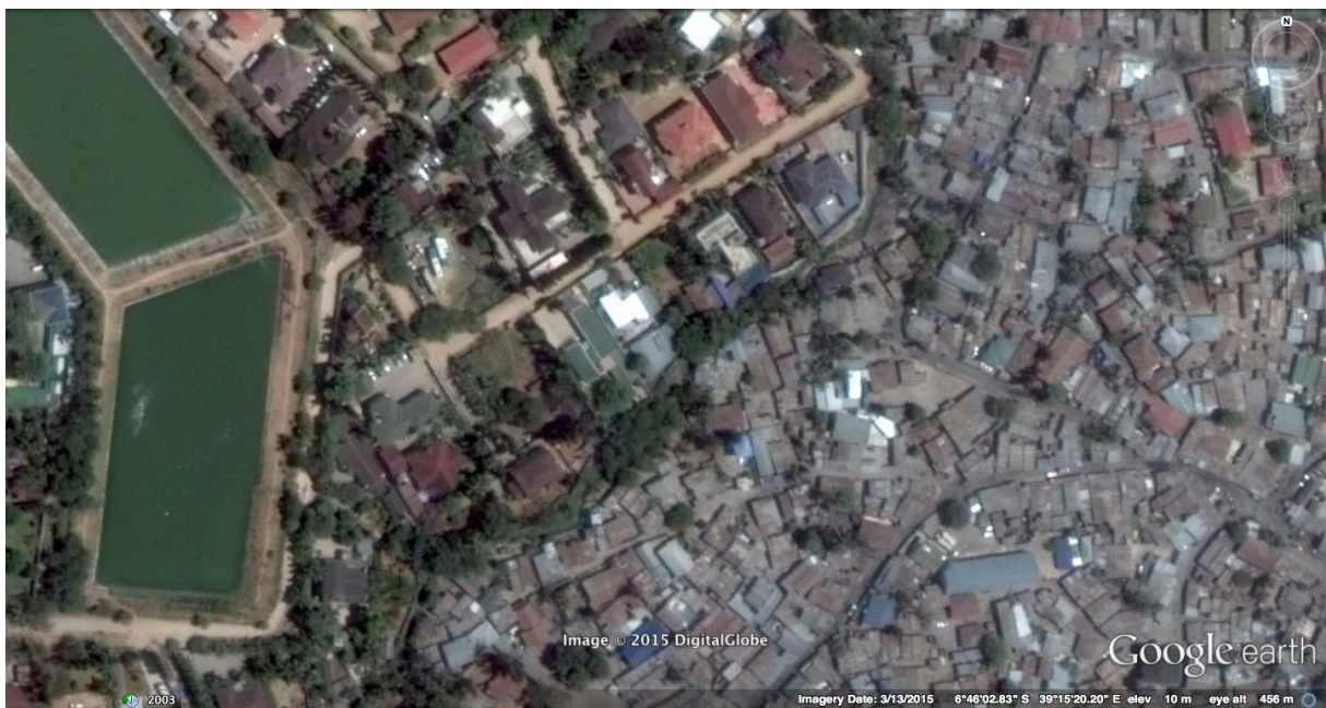
Figure 6. The waste stabilisation ponds and the contrasting “high income” and “low income” housing areas, narrowly separated by the Kijitonyama River
