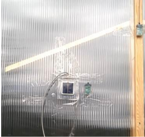
Figure 14. Placement of the SolData 881spc pyranometer and logger recording light intensity during measurement used for conversion from photometric intensity to radiometric irradiation.
