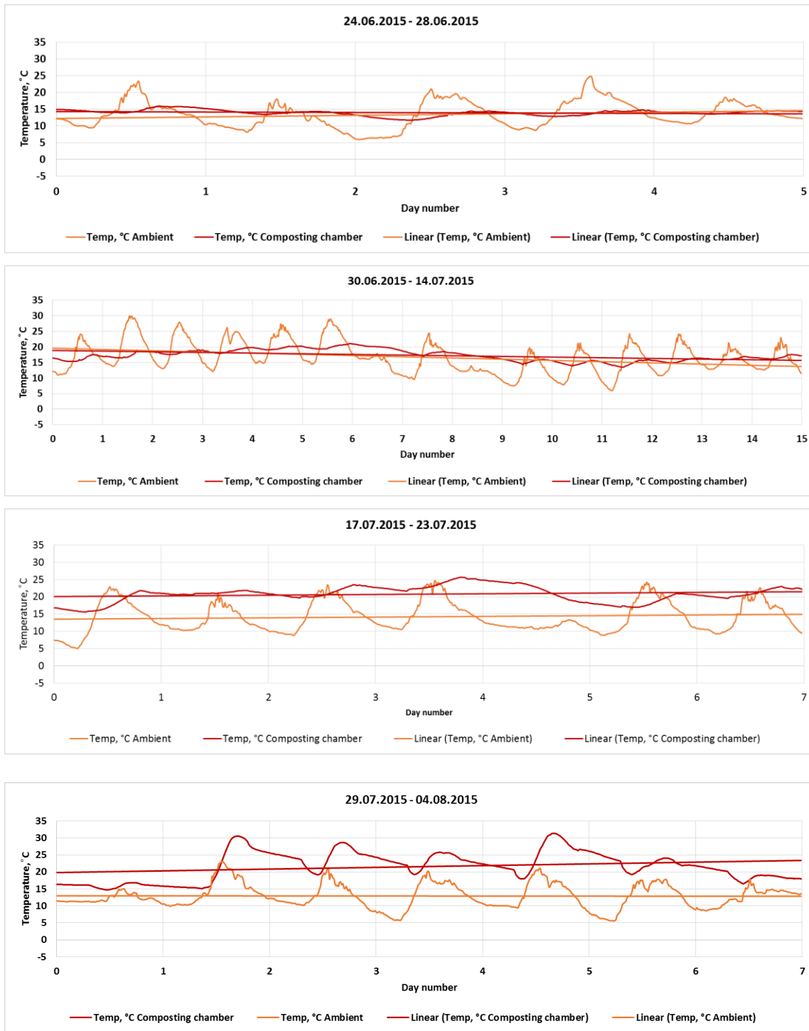
Figure 26. Temperature variation per period, comparison between the ambient temperatures and temperatures recorded in the composting chamber with trend lines to visualize the main trend in the temperatures over time and the average difference between the temperatures. The composting chamber temperature is higher in periods 1, 6 and 7
