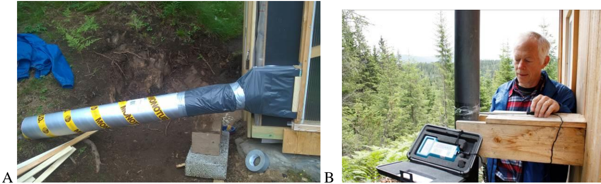
Figure 13. Air velocity measurement. A- The additional channel constructed to measure the air velocity at the inlet of the system. B – Measurements of air flow in the exhaust pipe
