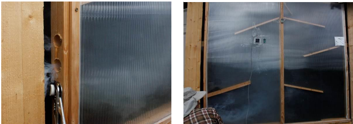
Figure 12. Testing with smoke pellets
