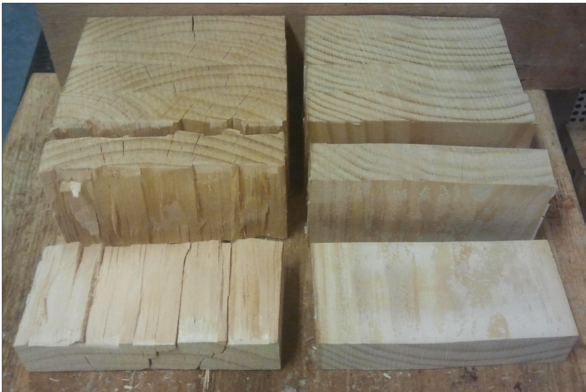
FIGURE 19: DELAMINATION TEST WITH GLUE LINES OPENED ON TWO MEMBERS. AT LEFT UNTREATED AND AT RIGHT ACETYLATED.
