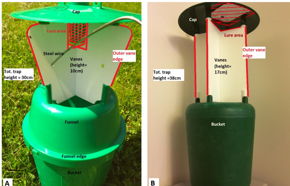
Figure 2 Pictures of the cross vane traps used in the different studies. A) Picture of the type of cross vane trap used in observations of Anthonomus rubi and Lygus rugulipennis behaviour. The cross vanes were of either green or white non-UV reflective plastic. B) Picture of the trap used in observations of Byturus tomentosus , with white non-UV reflective vanes.
