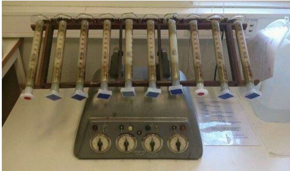
Figure 4. Automatic mixing rack used for SDS sedimentation test. (Photo-Yohannes B. Mekonnen).
