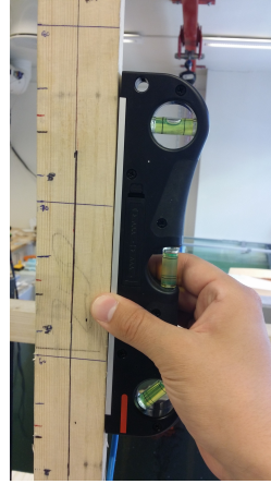
(b) Using a bubble level to ensure correct placement of sensor
