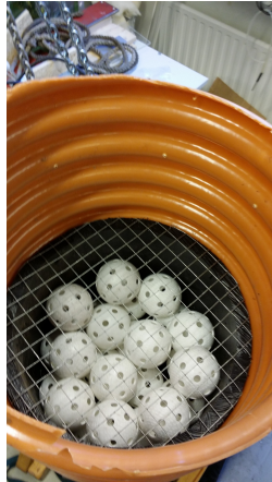
(b) 24 floorballs were inserted to break up the jetstream from the pump.
