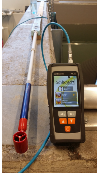
Figure 6: Instrument B. The MiniController MC20 and MiniWater ® 20 Mini.
