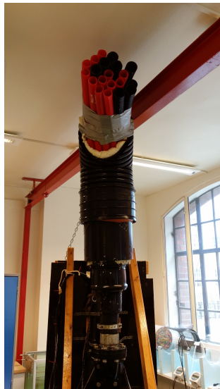
(g) Nozzle B connected to the pump.
