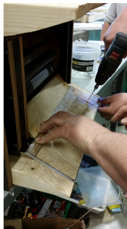
(c) Placing a smoother surface on the platform surface
