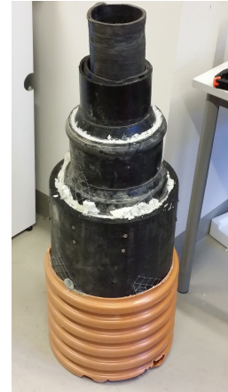
(d) All cracks were foamed to prevent leakage.
