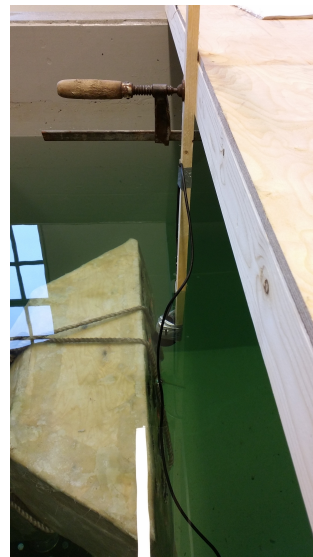
(b) Instrument A Taped to a Pole and Fastened to the Platform.
