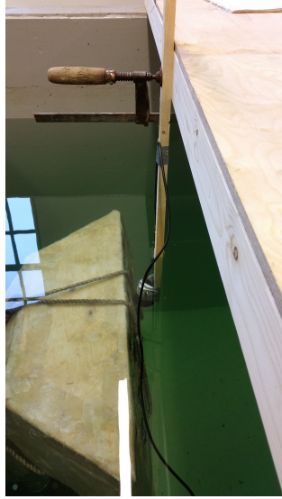
(a) The instrument 10 cm from the outlet and fastened to the platform.
