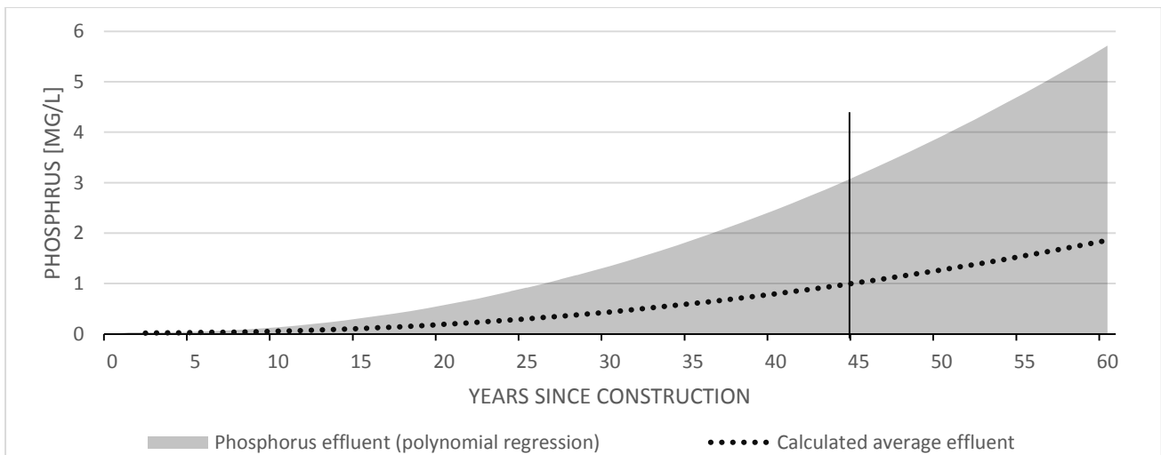
Figure 19, integral of the best fit (polynomial) regression (grey area), divided by number of years was calculated (dotted line). It was found that the average effluent would be 1 mg P/l after a lifetime of the filter of 45 years (black vertical line).
