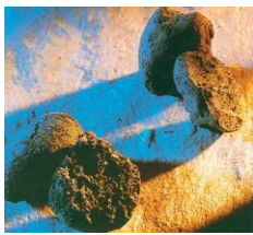
Figure 4. Filter media, Leca particles (weber SAINT-GOBAIN 2014)
