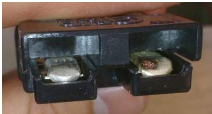
Figure 5.2: Contacts damaged by high current flow.
