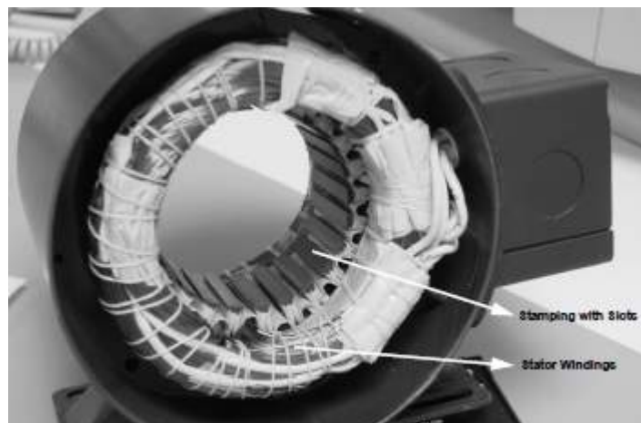
Figure 2.10: BLDC stator. Figure courtesy of Microchip [44].
