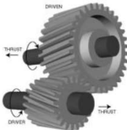
Figure 2.12: Helical gear. Figure courtesy of Martin Sprocket [39].
