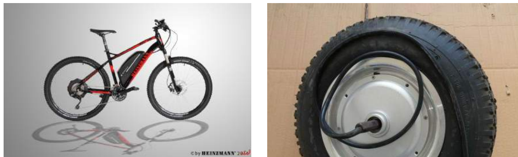
(a) E-bike with brushless motor. Image courtesy of Heinzmann . (b) Wheelbarrow motor. Image courtesy of alibaba.com
