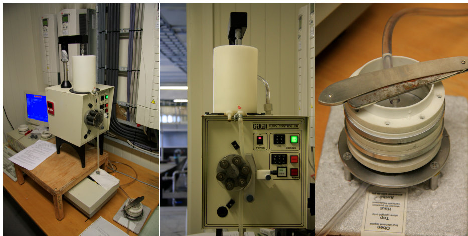
FIGURE 6: (LEFT) LASER SET UP WITH FLOWMETER GALAI CIS 1; (MIDDLE) FLOWCONTROLLER; (RIGHT) GAZE FILTER FOR CATCHING OUT-OF-RANGE PARTICLES
