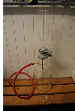
FIGURE 7: FILTRATION UNIT FOR TSS ANALYSES
