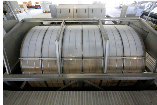
FIGURE 47: HDF 2006 WITH CHANGED FILTER PANEL – FROM 30 TO 10 \mu\text{m}
