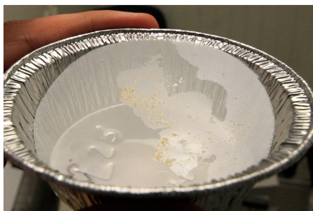
FIGURE 41: 300 \mu\text{m} FILTER GAZE FOR CAPTURING OUT.OF-RANGE PARTICLES. THE PRESENTED FILTRATE IS THE RESULTS OF A PSD ANALYZE OF THE EFFLUENT WATER FROM THE MBBR.
