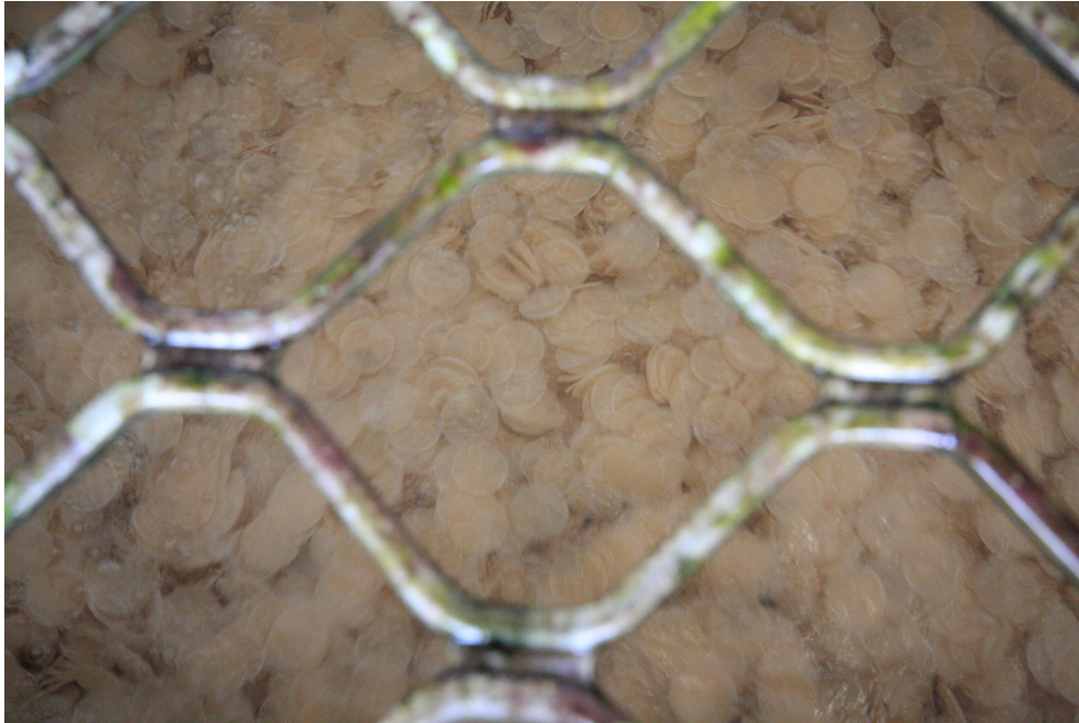
FIGURE 42: TOP VIEW INTO MBBR WITH MOVING BIO-MEDIA (KALDNES®BIOCHIP-P)
