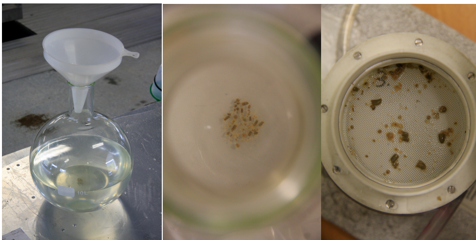
FIGURE 40: (LEFT) 5 LITER WATER SAMPLE TAKEN AT THE DRUM FILTER INLET. (MIDDLE) SEDIMENTED SOLIDS IN SAMPLE. (RIGHT) OUT-OF-RANGE PARTICLES AFTER LASER ANALYZE COLLECTED ON 600 \mu\text{m} GAZE.
