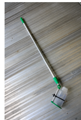
FIGURE 18: WATER SAMPLER. BOTTLE VOLUME: 1L
