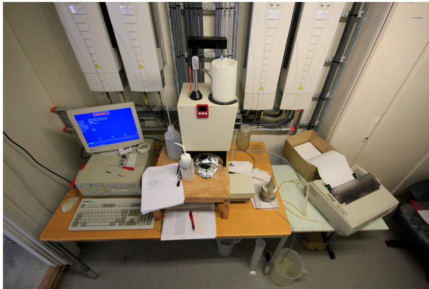
FIGURE 4: GALAI CIS-1 LASER SIZER SET UP INCLUDING FLOWMETER, PC AND PRINTER
