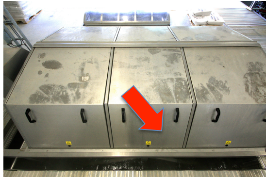
FIGURE 19: SAMPLE SPOT – DRUM FILTER INLET. THE RED ARROW MARKS THE SPOT, WHERE THE WATER SAMPLES WERE TAKEN
