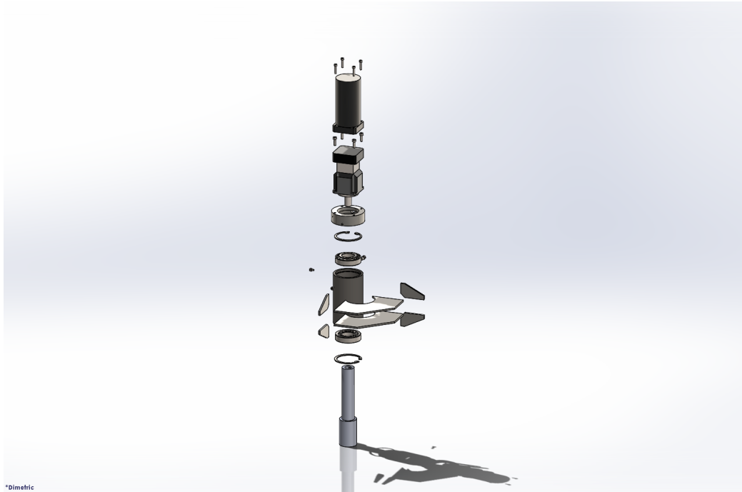
Figure 3.5: An exploded view of the steering components [Blomberg, 2014].
