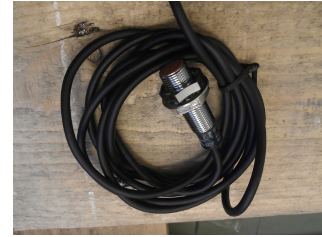
(c) The 24 volt inductive sensor chosen for absolute position measurements of the steering axle.
