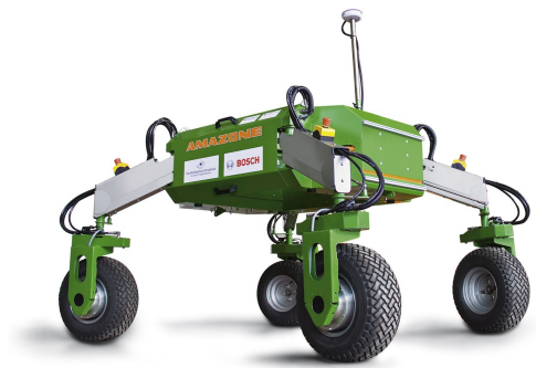
(a) BoniRob is a multi directional mobile robot that uses the app-concept by allowing different tools to be added or removed as needed. The track width of BoniRob is adjustable [Biber, 2014].
