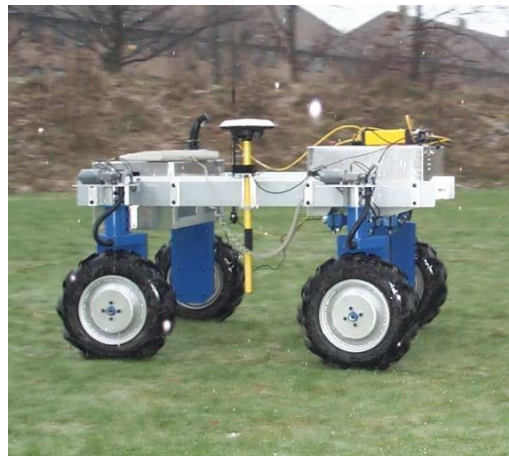
(d) Mobile Robot for weeding is one of the first attempts on designing a autonomous mobile agricultural robot [Madsen and Jakobsen, 2001].
