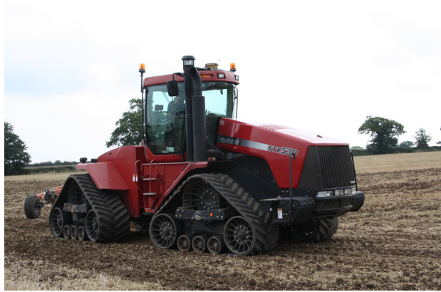
Figure 3.2: Articulated steered modern Case IH STX 530 Quadtrac at the Maldon Working day 2011, courtesy tractors.wikia.com.
