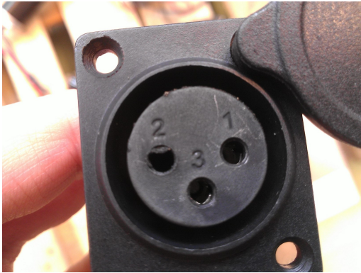
(a) Shows the damaged battery XLR-plug
