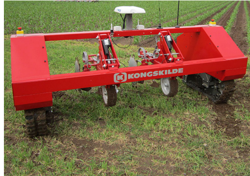
(b) Robotti is a electric tracked autonomous agricultural robot that uses various demountable implements, intended for plant production [Green, 2013].
