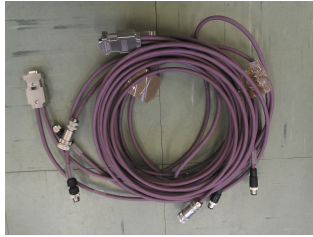
(a) CAN bus-cable custom made for our robot that all the motor controllers and the laptop is connected to.
