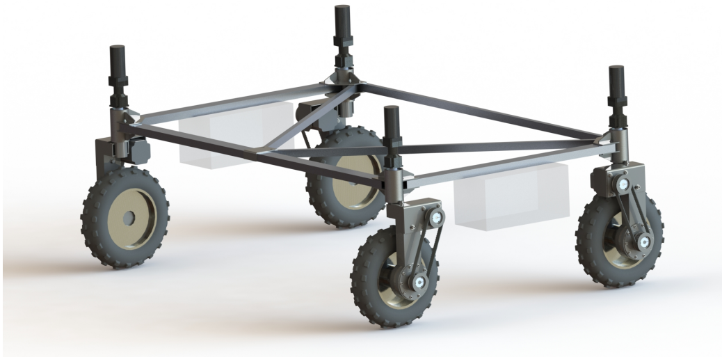
Figure 6.4: This figure shows a rendering from SolidWorks of the frame showing the tool replica as the triangle in the middle of the robot [Blomberg, 2014].
