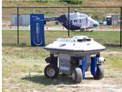
Figure 3.3: Four wheel steered Seekur is a all-weather, outdoor robot platform for outdoor research, courtesy Adept MobileRobots
