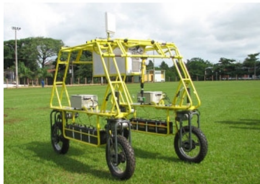
(c) Agricultural Mobile Robot is intended for for long operation time while collecting agricultural field data [Tabile et al., 2011].
