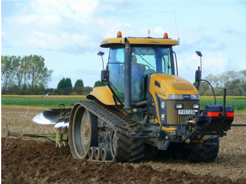
Figure 6.1: Normally when ploughing, either the left or right wheel pair tracks the exposed furrow, and this amplifies soil compaction. The tractor shown above has both wheel pairs on the unploughed land, and this reduces soil compaction to some extent [Bjugstad, 2014]. A Caterpillar Challenger MT765B tracked tractor at work ploughing a field near to Leverton Lucasgate, Lincolnshire, Great Britain. The photo was taken on 22 October 2008.[Billinger, 2008].
