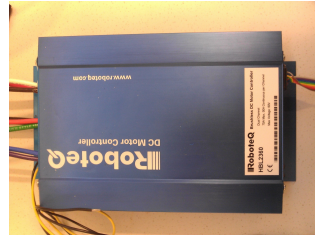
(c) The versatile Roboteq HBL2360 motor controller for the propulsion motors
