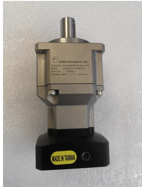
(b) The APEX DYNAMICS AB060 two stage planetary gear with 60:1 ratio chosen for the servo motors.
