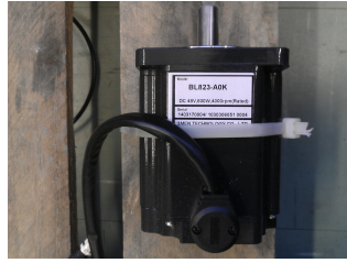
(b) The chosen propulsion motor BL823-A0K from 3MEN TECHNOLOGY in Taiwan
