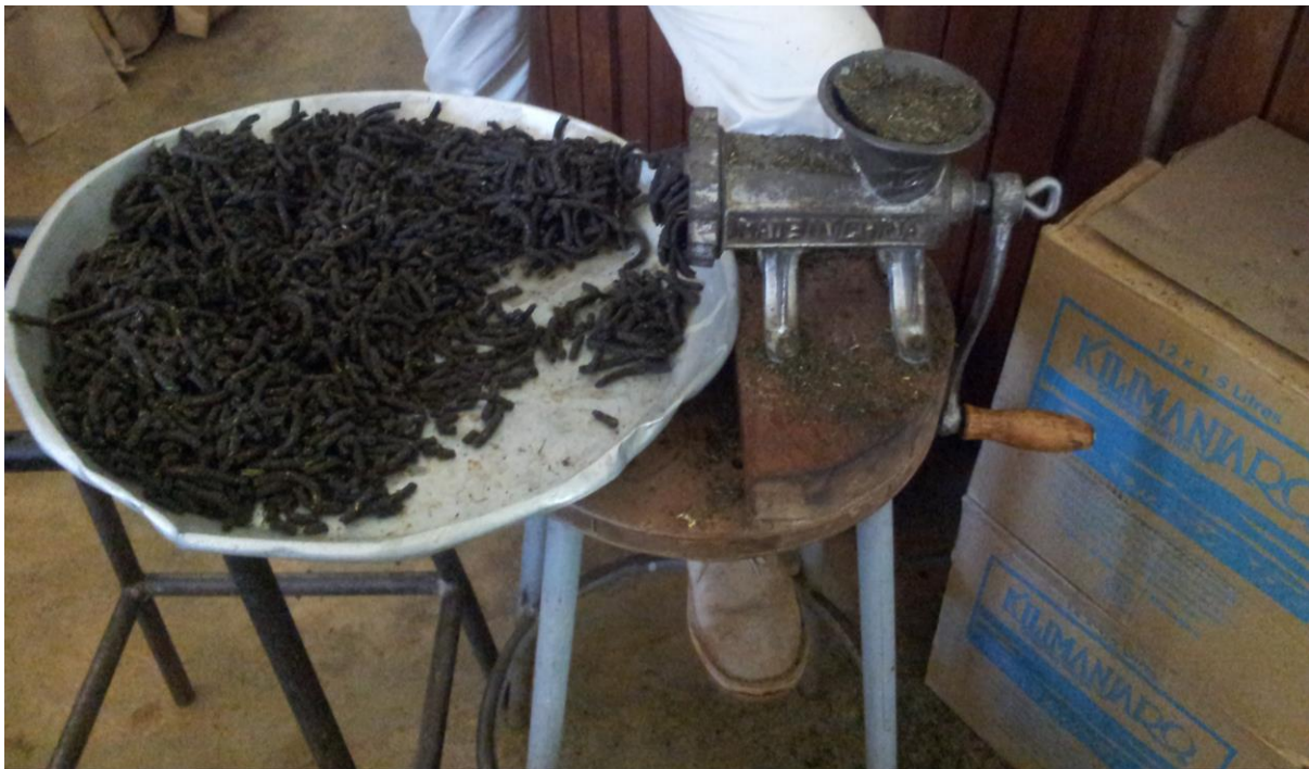
Fig. 3. Manufacturing of the pellets manually performed with a meat grinder
