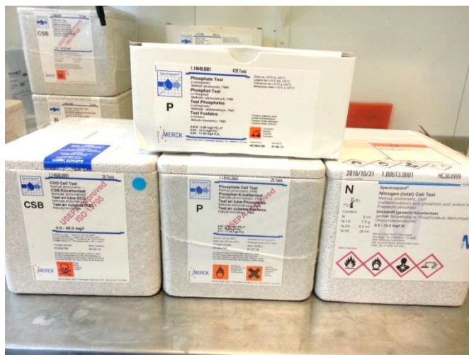
Figure 4: Test kits used to quantifying COD, TP, TN and PO 4 -P
