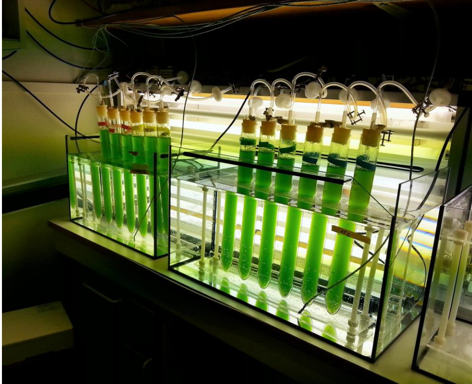
Figure 6: Illustration of photobioreactor-systems used in all the experiments. Note that the water exchange system (temperature control) is absent, unlike the systems used in the daylight- and high light exposure experiments. In illustration above, temperature was controlled by keeping a stable room temperature and heating cobs. M. Evjen, 2014.
