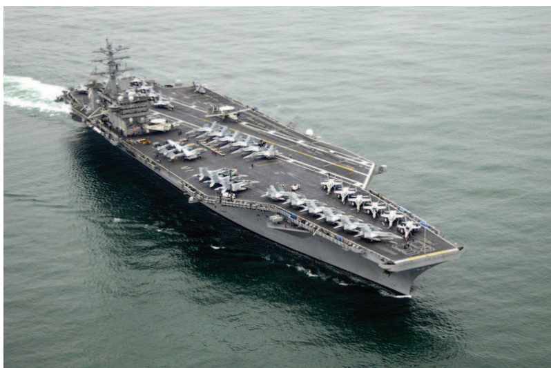
Figure 7: USS Nimitz Aircraft Carrier commissioned in 1975. (9) USS Nimitz is propelled by: - 2 x Westinghouse A4W nuclear reactors - 4 x Steam turbine - 4 x Shafts - Total power: 194MW
