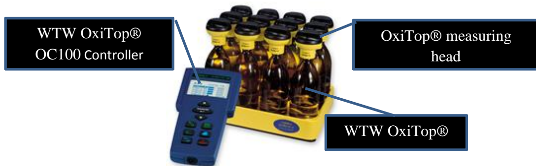
Fig. 10: OxiTop system “WTW OxiTop® OC100” components for biochemical oxygen demand (BOD) test (WTW, 2014).
