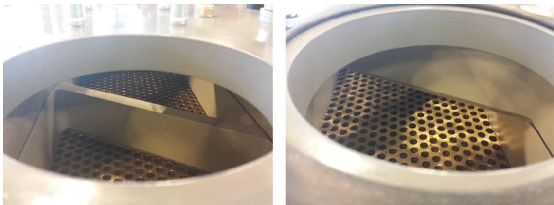
Figure 23: When looking through two of the holes in the top, we can clearly see that the diagonal splitter in the frame, no longer will restrict the water from filling the total area.
