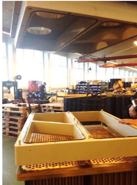
Figure 22: The original frame still mounted on the top part which is lifted off, and an extra flow frame is inserted in between.
