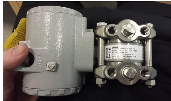
Figure 16: The pressure transmitter where the two blue tubes from Figure 15 are connected. This is a spare unit. The symbol from the flow chart is to the right.
