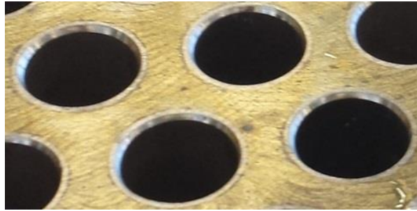
Figure 29: Close up picture of the pipes fastened to the plate holding them.
