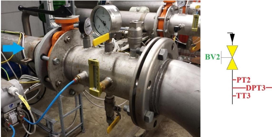
Figure 14: A close up picture of the area where the pressure sensors are fitted, as well as the temperature sensor. The blue arrow represents the flow direction, and to the right are the symbols used in the flow chart.
