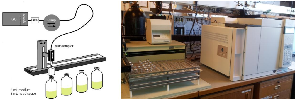
Figure 3.2 Gas chromatograph (GC) and autosampler. To the left is a schematic overview of the autosampler and the GC, to the right is a photograph of the setup. The photograph shows the autosampler with its arm to the left, the pump is on top of the autosampler and the GC is to the right side. The flasks are in a rack giving known positions for the robot to sample from. Helium is fed through the pump. (The figure is modified from that found in Molstad et al. 2007)
