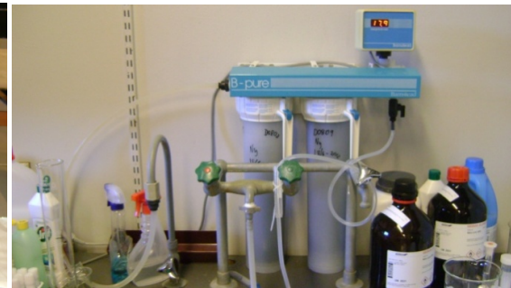
Double deionization unit for water purification
