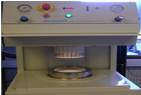
Sample hanging in Ultra-clave after digestion
