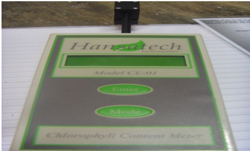
Figure 7. Hansatech CL-01-chlorophyll content meter (Hansatech Instruments, King's Lynn, Norfolk) used to measure chlorophyll content in leaves.
