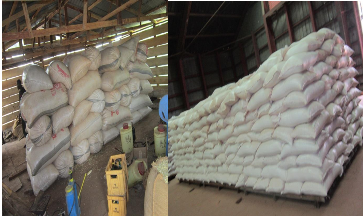
Figure 12: An improved traditional storage method (S2)
