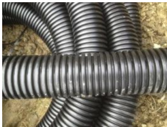
Photo: 24 Perforated drainage pipe
