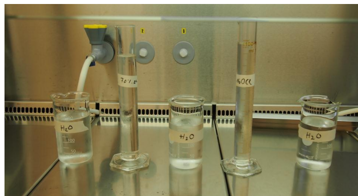
Figure 3.4 Set up for surface sterilization of wheat leaves. From left: 100 ml distilled water, 50 ml 70 % Ethanol, 100 ml distilled water, 50 ml 0.5 % NaOCl, 100 ml distilled water. Photo: A. Ruud 2012
