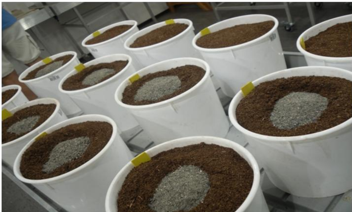
Figure 9: Different treatments containing sand, peat, R1 and R2 in pots before mixing
